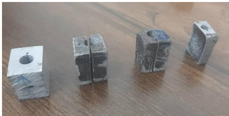
Figure 6. The compression samples cut from the central area of the MAF samples
