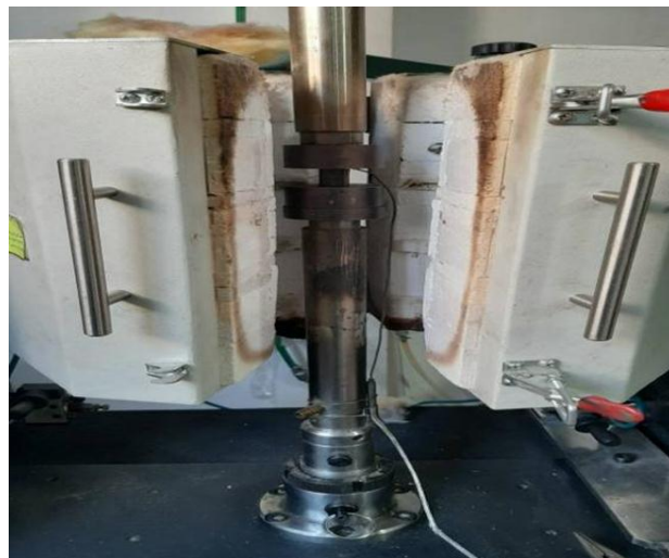
Figure 3. Resistance furnace equipped with a thermometer of the SANTAM tensile-compression machine
