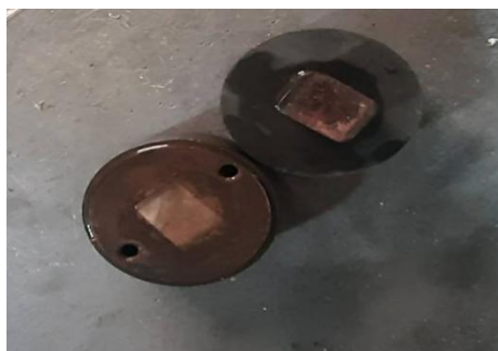
Figure 4. Complete and optimal filling of the mold after each load application cycle
