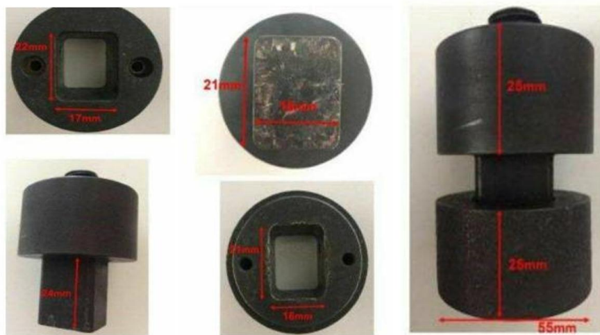
Figure 1. Picture of the MDF mold used in this study
